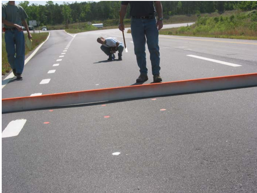
Figure 2.3 Demonstration of Manual Measurement of Rut Depth
