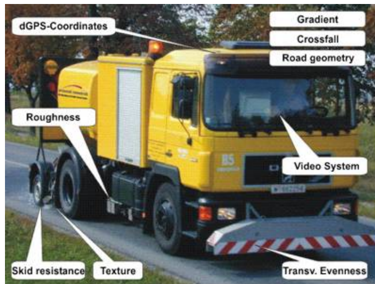
Figure 2.11 The RoadSTAR Transverse Evenness Measuring Device
