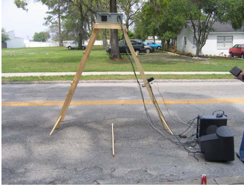
Figure 3.9 Installation of the Frame and the Scanner
