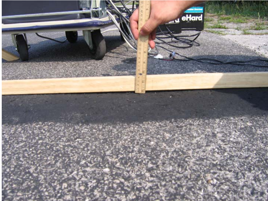
Figure 5.8 The Manual Measurement of the Left Rut Depth
